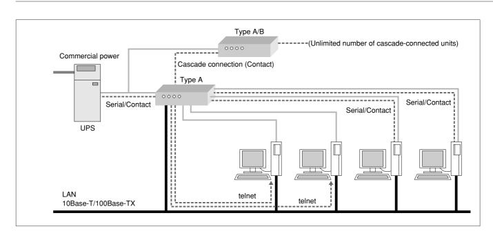
Fig. 3 System Configuration Example (Type A)
